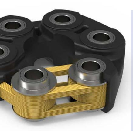
Torque is transmitted almost exclusively via the vulcanised-in cord inlays (Tenpu® fiber technology) by the unique SGF tension-force-principle.
